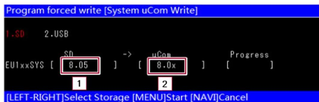
— If the SD version is displayed as “- - - - -”, the data on the SD memory card or microSD card may be corrupted. Please repeat the firmware download and installation process.
