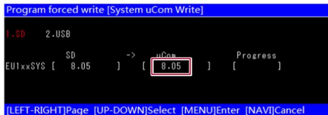
**12. Eject the SD memory card or microSD card on the “Program forced write [System uCom Write]” screen and turn the vehicle’s key to OFF position to power off your navigation system.**
