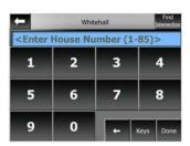
Although QWERTY-type keyboards also contain number keys, when entering a house number, the program offers the more convenient numeric keypad.
