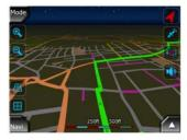
The line of the route is displayed on the driving side of the road for two-way and on the axis in case of one-way streets. When the map is zoomed in and the line is wide enough, small arrows show the direction of the route. This can be useful if you preview the route before starting the journey or when entering a complex junction.
