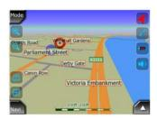
Note: When your GPS position is available, and Lock-to-Position (Page 27) is active, the cursor is the current GPS position, the red arrow. When you select another point by tapping the map, or using the Find menu (Page 62), the new Cursor is shown on the display with the red dot and the radiating red circles.
