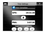
Turn on the Auto Correction switch to let AVIC-S2 frequently check and correct the internal clock with the GPS time.
