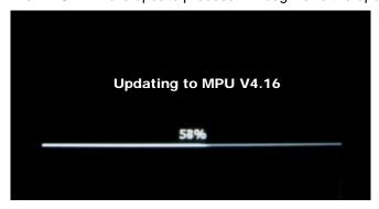
**WARNING!** While your AppRadio is being updated, **DO NOT** turn off the power to the system. Severe damage to your AppRadio multimedia system could result from your failure to obey this warning.
