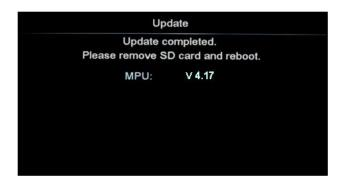
8. Eject the microSD card from the AppRadio and press the reset button. Your AppRadio is now ready for use.
