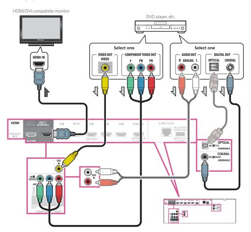
• With factory default settings, video from the video cable or component cable will not be output from the HDMI terminal. To output video, you must switch video input to the device connected with the video cable or component cable and set **V.CONV** to **ON** (page 69).
