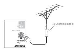
To improve AM reception, connect a 5 m to 6 m (16 ft. to 20 ft.) length of vinyl-coated wire to the AM LOOP terminals without disconnecting the supplied AM loop antenna.
