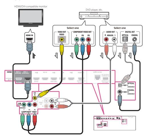
• With factory default settings, video from the video cable or component cable will not be output from the HDMI terminal. To output video, you must switch video input to the device connected with the video cable or component cable and set **V.CONV** to **ON** (page 69).
