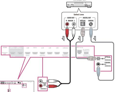
If your turntable has line-level outputs (i.e., it has a built-in phono pre-amp), connect it to the ANALOG IN 1
