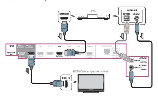
— If you use a digital audio cable or RCA (analog) audio cable, you'll need to tell the receiver which digital input you connected the set-top box to (see The Input Setup menu on page 40).
