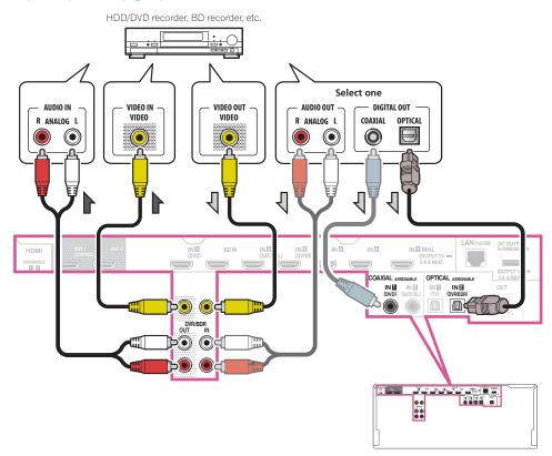
In order to record, you must connect the analog audio cables (the digital connection is for playback only) (page 88).
