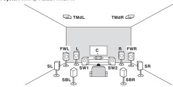
A 9.2 ch surround system connects the left and right front speakers (L/R), the center speaker (C), the left and right top middle speakers (TMdL/TMdR), the left and right front wide speakers (FWL/FWR), the left and right surround speakers (SL/SR), the left and right surround back speakers (SBL/SBR), and the subwoofers (SW 1/SW 2). Dolby Enabled Speaker can be used for the top middle speakers (page 24).
