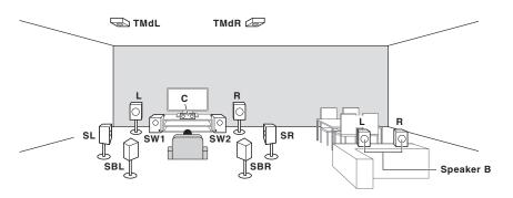
With these connections you can simultaneously enjoy 7.2-channel surround sound in the main zone with stereo playback of the same sound on the B speakers. The same connections also allow for 9.2-channel surround sound in the main zone when not using the B speakers.
