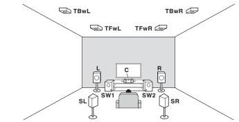
A 9.2 ch surround system connects the left and right front speakers (L/R), the center speaker (C), the left and right top forward speakers (TFwL/TFwR), the left and right top backward speakers (TBwL/TBwR), the left and right surround speakers (SL/SR), and the subwoofers (SW 1/SW 2).
