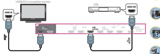
• Even if your set-top box is equipped with an HDMI output terminal, in some cases the sound is output from the digital audio output (optical or coaxial) and only the video is output from the HDMI output terminal. In this case, make the HDMI and digital audio connections as shown below.
