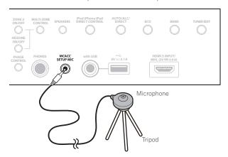
If you have a tripod, use it to place the microphone so that it's about ear level at your normal listening position. If you do not have a tripod, use some other object to install the microphone.
