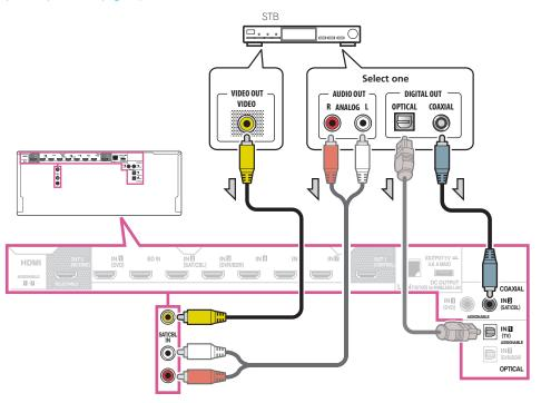
• If your set-top box is equipped with an HDMI output terminal, we recommend connecting it to the receiver's **HDMI SAT/CBL IN** terminal. When doing so, also connect the receiver and TV by HDMI (see <u>Connecting using HDMI</u> on page 26).
