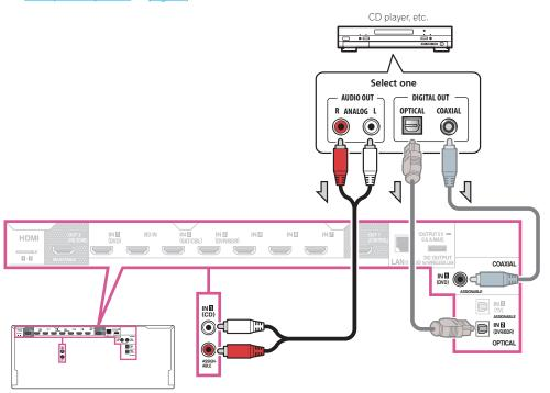
If your turntable has line-level outputs (i.e., it has a built-in phono pre-amp), connect it to the ANALOG IN 1
