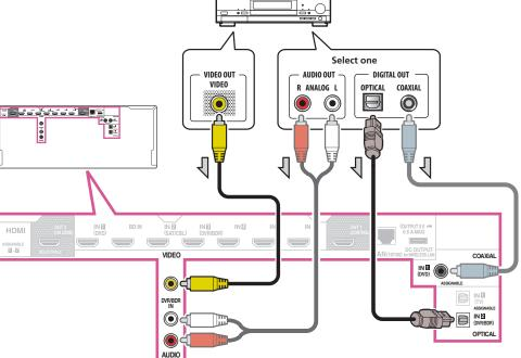
• If your HDD/DVD recorder, BD recorder, etc., is equipped with an HDMI output terminal, we recommend connecting it to the receiver's HDMI DVR/BDR IN terminal. When doing so, also connect the receiver and TV by HDMI (see Connecting using HDMI on page 26).
