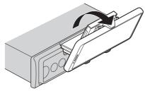
The holder angle range: Downward 45° to upward 100°
